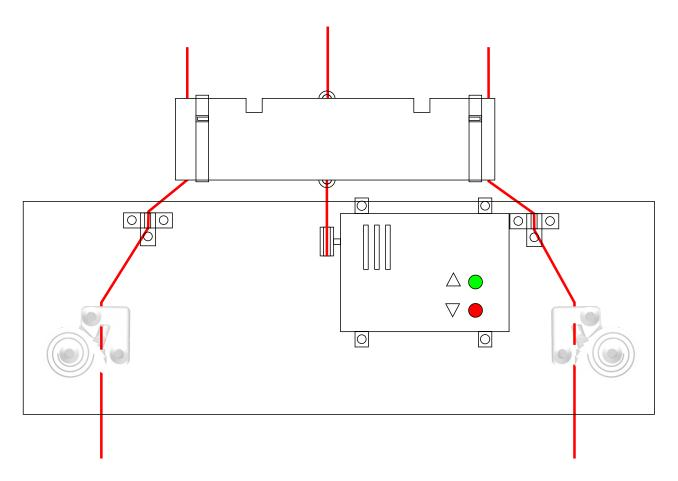
Use Brackets on the bottom of the firing point target changer board so that the board lips over the back of the table. Use a gclamp or similar to stop them being knocked off by the shooters
